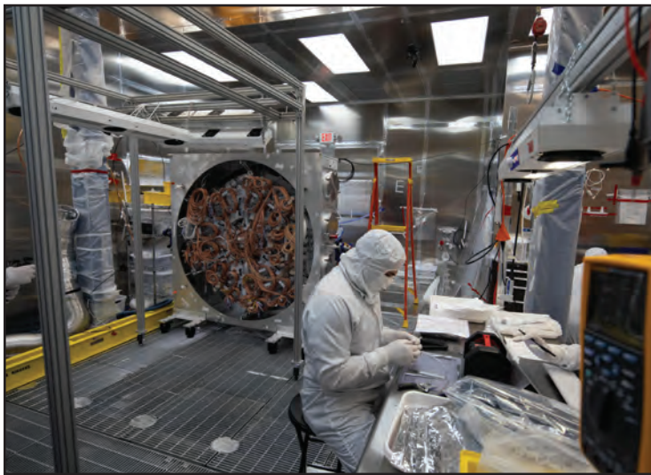
Top: The rear of one of the photo-multiplier tube (PMT) arrays for the LZ dark matter detector.
