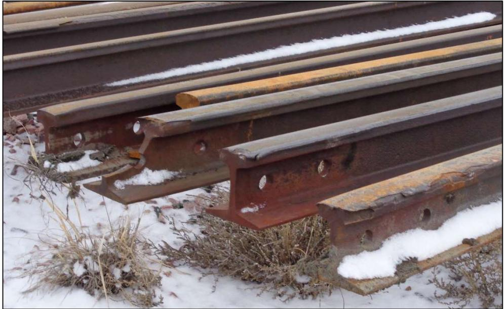
Typical rail end wear, rail from PRC main line west of Ft. Pierre
