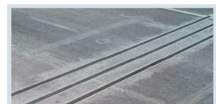
In-pavement sensors detect tire inflation at 75 mph.
