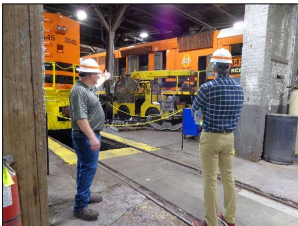
Photos showing deficiencies in current roundhouse: On left, note very limited vertical clearance between top of locomotives and wood roof rafters. Also note portable small crane, required due to lack of adequate overhead bridge cranes. On right, note very limited side clearance between locomotive and wall, and lack of work platforms at the level of the locomotive side walkways.
