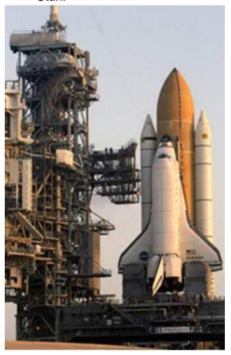
The engineers who designed the SRBs would have preferred to make them a bit larger, but the SRBs had to be shipped by train from the factory to the launch site. The railroad line from the factory happens to run through a tunnel in the mountains and the SRBs had to fit through that tunnel.
