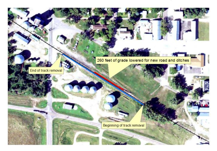
The red line indicates the grade lowering for the new road with ditches is approximately 260 feet. The blue line indicates 500 feet of track removal.
