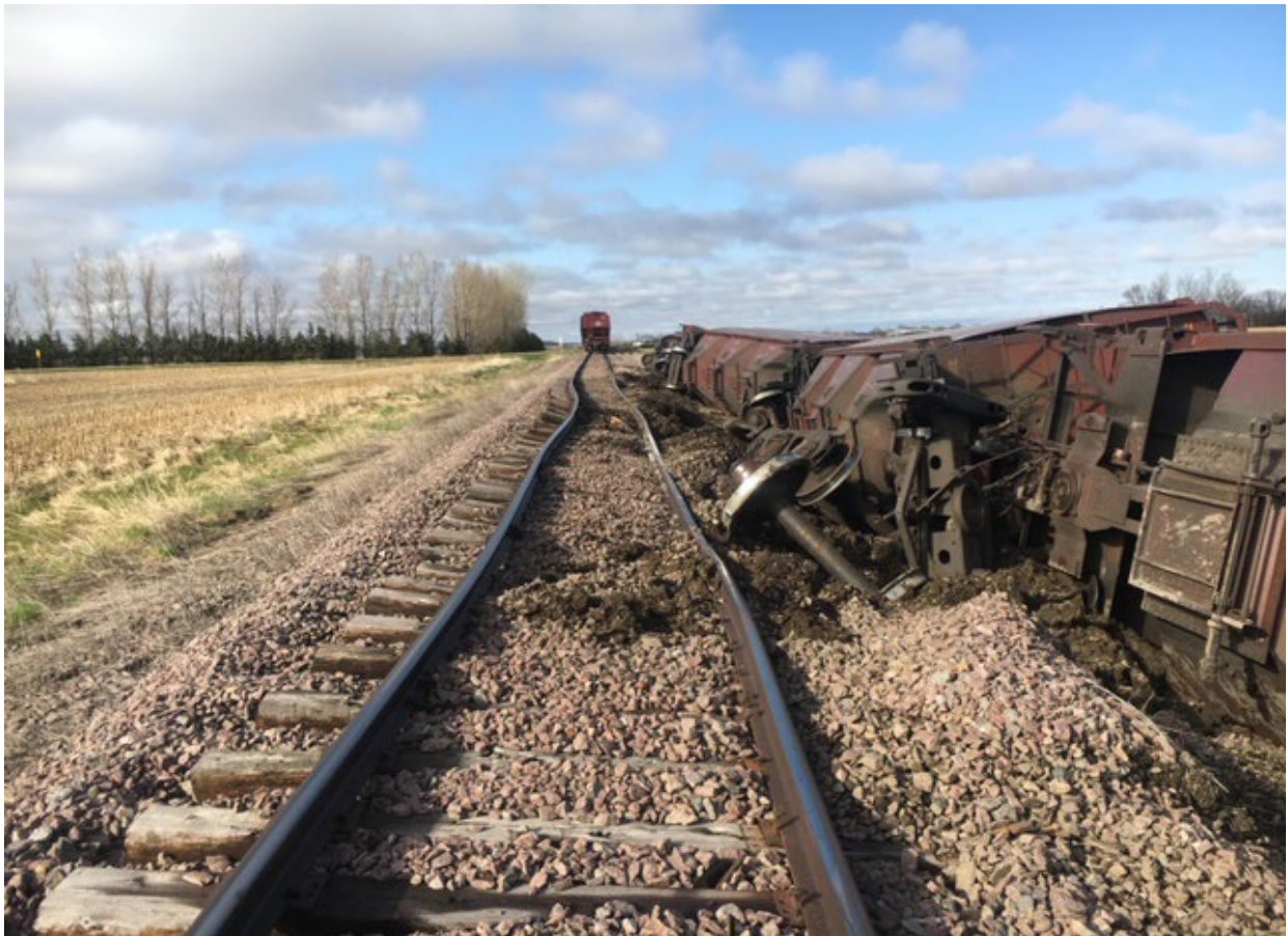
2020 Derailment – soft subgrade/poor tie condition
