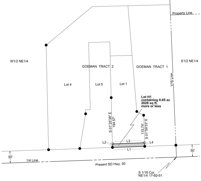
Note: The coordinates, distances and areas shown on this plat are based on the South Dakota State Plane coordinate System - South Zone NAD 83/11 epoch 2010.00 Geoid 12A SF = 0.9999570042
