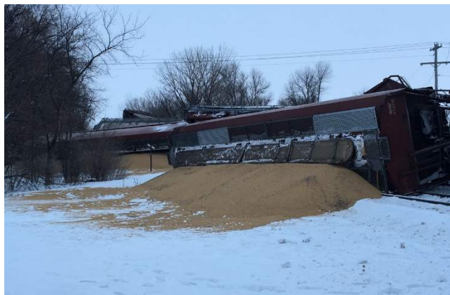
Figures 1, 2, & 3 – Previous derailments caused by rail defects.
