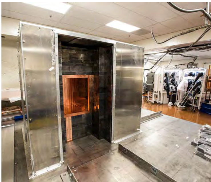
Top: Once complete detectors for the MAJORANA DEMONSTRATOR will slide into a multi-layered shield.
