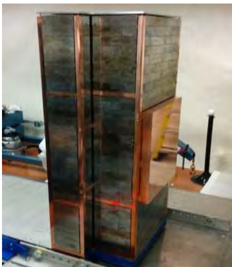
Fig. 3 Lead shield installed on MJD blank monolith.
