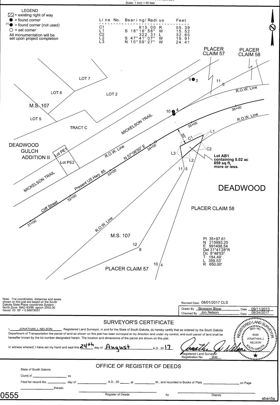
in a portion of the 66 foot right-of-way of US Highway 85 in Placer Claim 58 in Section 27 - Township 5 North - Range 3 East of the B.H.M., located in the City of Deadwood
